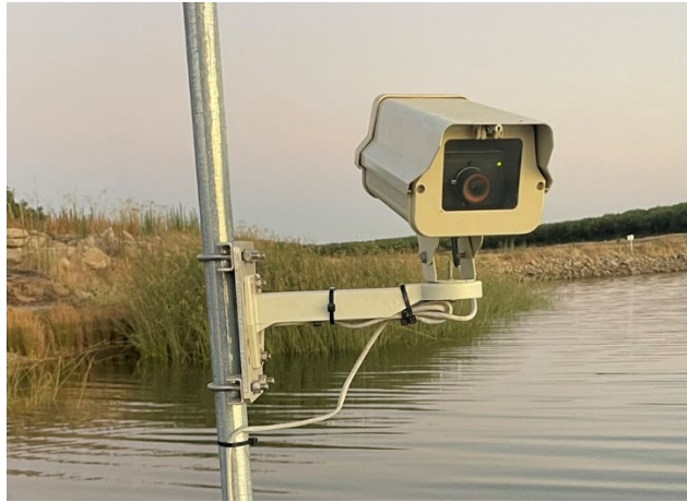
Figure 15. PhenoCam Installed at EC Station
