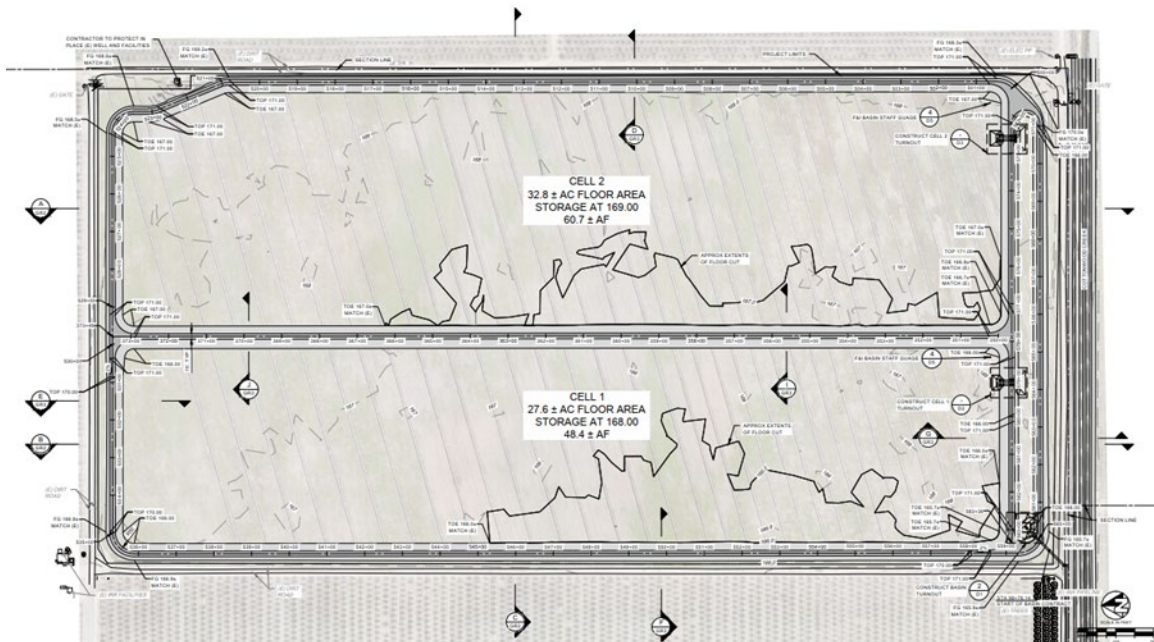
Figure 10. Groundwater Recharge Basin Site Plan
