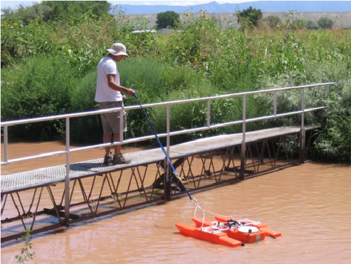
Figure 2. Photograph of an ADCP Measurement Using the Riverboat
