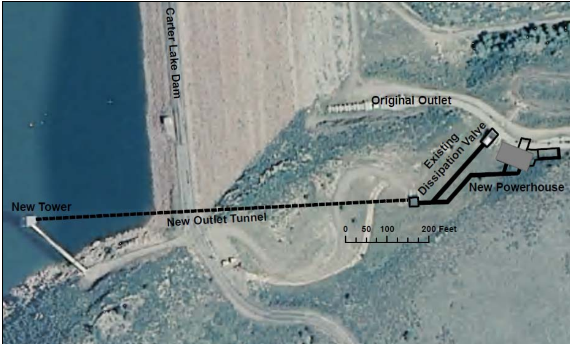
Figure 2. Layout of Project Facilities
