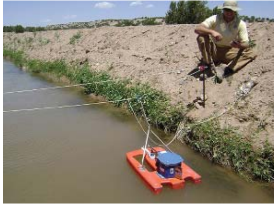
Figure 2. Bank-operated rope and pulley system with operator and ADCP
