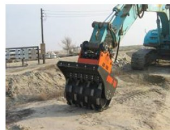
Figure 5. MBW 36" vibratory roller attached to the end of an excavator arm.
